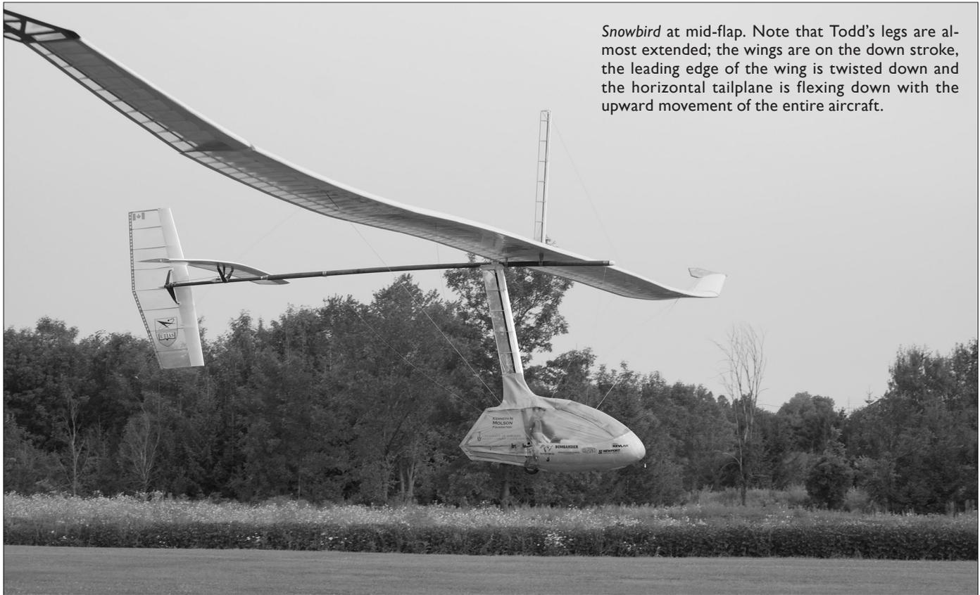
*Snowbird* at mid-flap. Note that Todd's legs are almost extended; the wings are on the down stroke, the leading edge of the wing is twisted down and the horizontal tailplane is flexing down with the upward movement of the entire aircraft.
