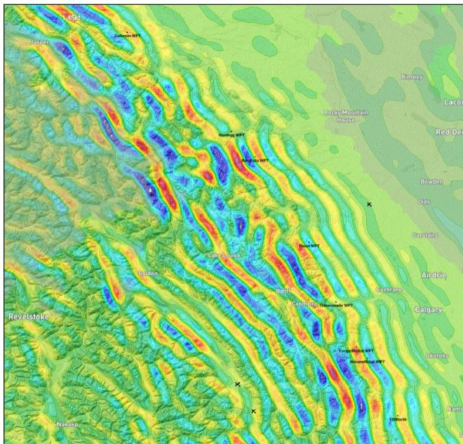
*Wave forecast from skysight.io – red is lift, blue is sink. After a flight is over, you can import your .igc file and see how accurate the forecast was. You can also create waypoints directly on the forecast map. Pro tip – don't put your turnpoints in the sink.*
