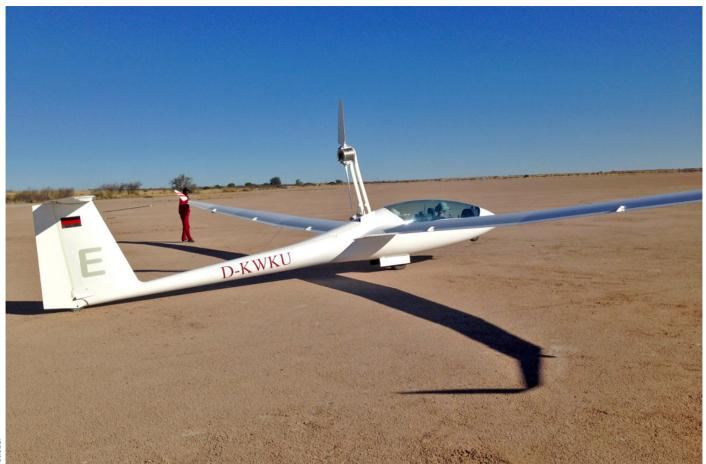
The Arcus E is ready to launch. The 40 KW (53 hp) electric motor in the propeller hub provides good take-off performance at maximum gross weight.
