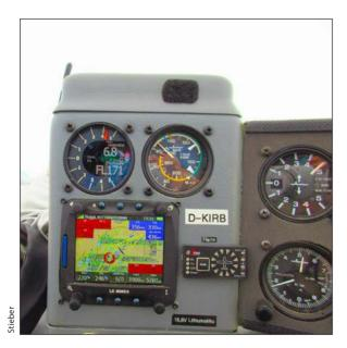
The panel in the picture is from an EB28 (Super ASH-25) which an old Akaflieg buddy of mine had stationed in Bitterwasser for the winter. The LX Vario shows the plane at Flight Level 171 (altimeter shows 5170 meters), climbing with an average of 6.8 m/s which is nearly 14 kts. It came from the Bitterwasser website. Basically a snapshot of what conditions can be there.
