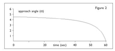
Figure 2 shows a glider flying a 5° glide angle to the destination point. Time is in seconds to 60 seconds, which represents a final approach of 5064 feet along the approach path to the destination point. The curve shows the angle  $\alpha$  down to the undershoot reference point as the glider converges on the destination point. Below are some points from the graph and corresponding distances and altitudes.
