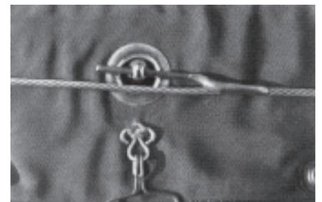
This pin is not far enough in. With more handling and movement of the canopy container, it will work loose.
