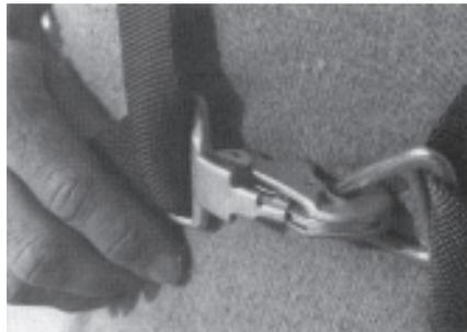
Quick-release buckle used on many chutes. This one is not fully closed and could release if snagged. Push release lever all the way down until it "clicks".
