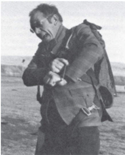
Fig. 3 John would have to pull more than 300 pounds to dislodge the bent ripcord pin from the metal cone.
