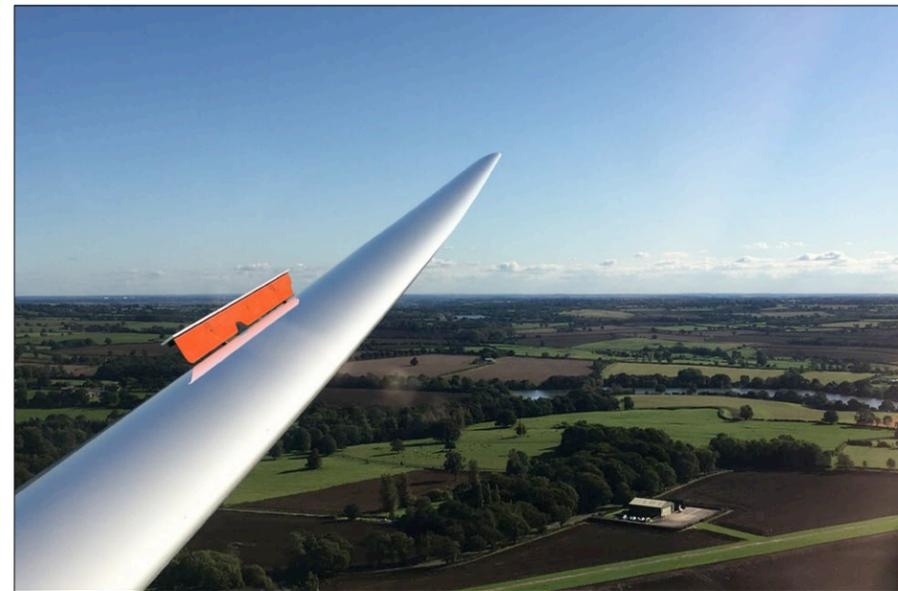
Above: *Winching* – Once in the full climb on a winch launch, briefly look along either wing to check you are at a suitable angle of climb, the amount of 'lay-off' to compensate for a cross-wind element if appropriate, and for any other issues.
