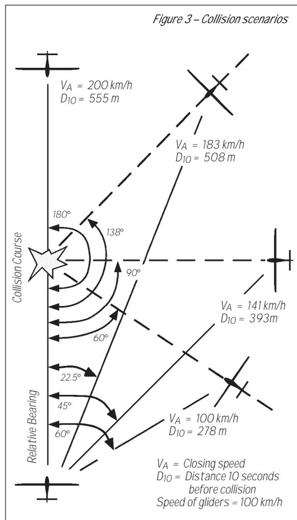
tion so dangerous is the unexpectedly high closing speed. Although both gliders fly only at 100 km/h, they are also closing on each other at 100 km/h, or over 100 ft/second, just as if they were flying head-on into a brick wall! With more acute convergence angles, closing speeds decrease significantly.
