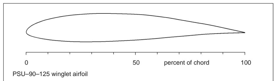
at negative  $C_l$ 's, so that sideslips and horizontal gusts can be tolerated. The corners of the laminar bucket have been rounded to avoid unstable yawing moments that would be generated otherwise if the sailplane yawed to angles exceeding those corresponding to the sharp corners of the traditional Wortmann sailplane airfoils. Finally, the airfoil was designed to avoid laminar separation bubbles down to  $Re = 350,000$ ."
