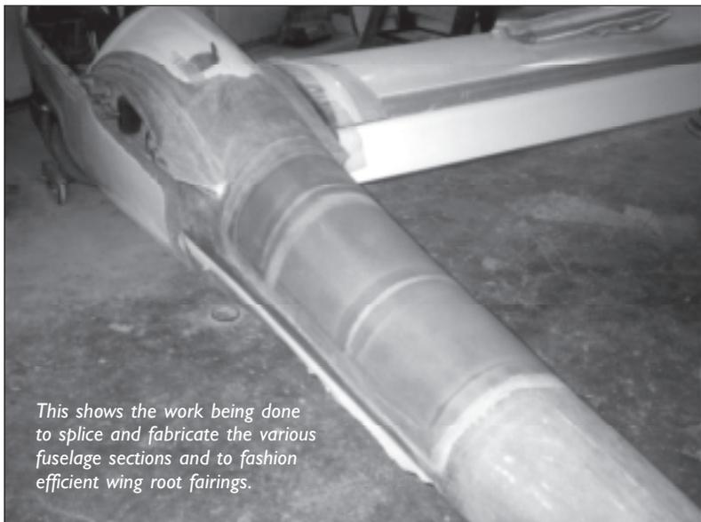
*This shows the work being done to splice and fabricate the various fuselage sections and to fashion efficient wing root fairings.*
