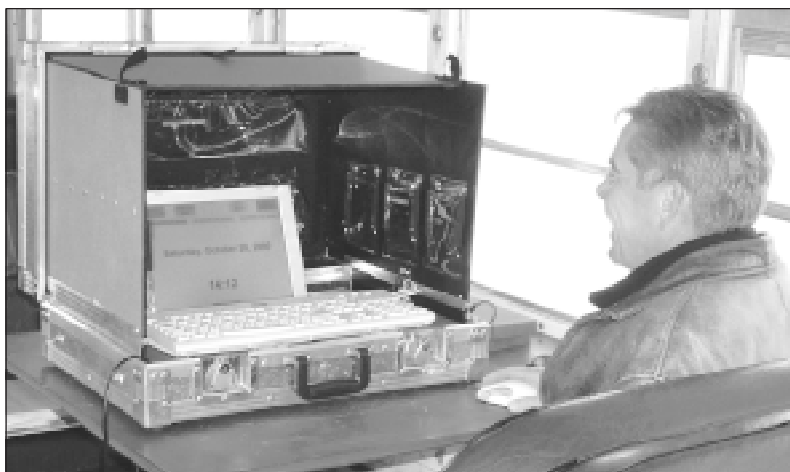
Figure 3 Flightline computer system housed in its case and in use at SOSA's flightline bus. The weight is about 30 lbs, and closed case size is 20" x 30" x 6".
