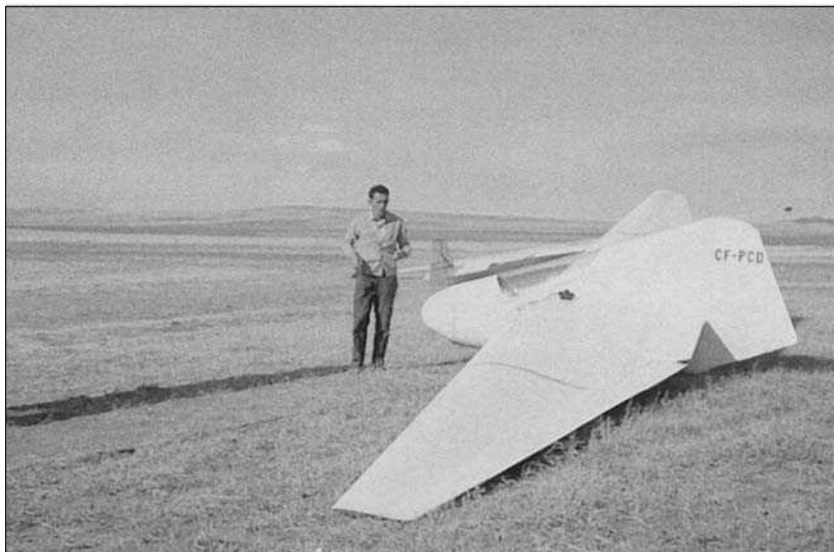
1965 – Mike Kiss of Calgary likes to build and modify his birds. This modified AV-36 shows a streamlined canopy design from nose to fuselage. It took a small pilot to fly the sleek looking ship.
